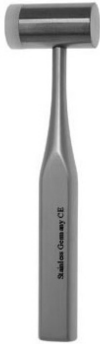
G20-30 Combination Mallet 7 1/2", 8oz (227g), Head Stainless Steel, With One Nylon Cap 25mm, Aluminum Handle
